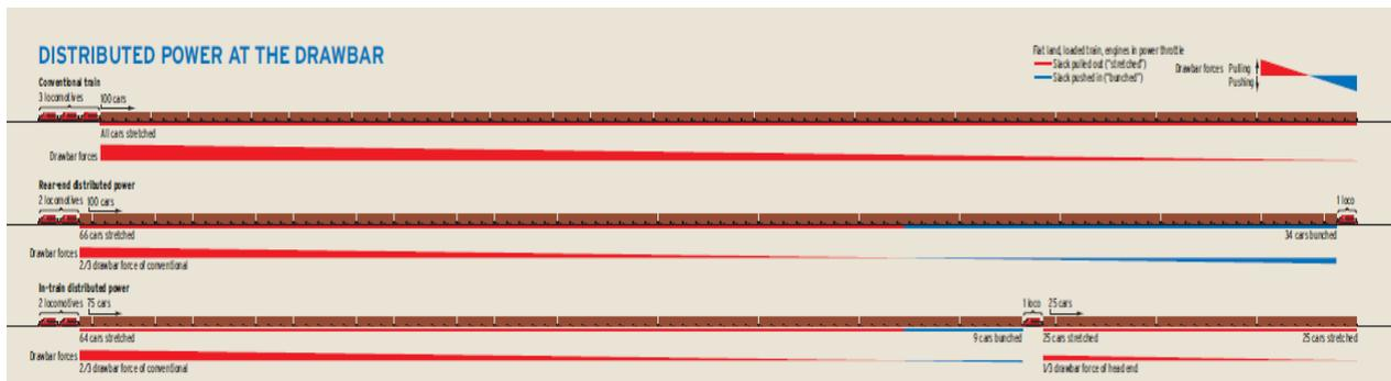
would be required if all the power exerted were at the head end. On an undulating track profile, a skillful engineer can manipulate the relative power outputs, dynamic and air brake applications to minimize run-in and run-out of the coupler slack throughout the train.
